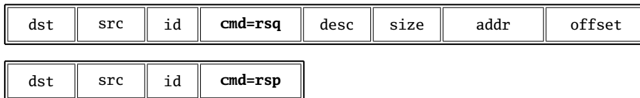
Figure 8.17 – Formats of read-stream Messages. The destination field (dst) encodes the address of the stream controller to which the message is delivered; the source field (src) encodes the source address of the sending module. The identifier field (id) encodes an identifier that associates request and response message pairs. The stream descriptor register is encoded in the descriptor field (desc). The size field (size) encodes the number of records to be transferred. The address field (addr) encodes the address to which records are transferred; the offset field (offset) encodes the offset that is used to compute the effective addresses of the records comprising the stream transfer.
