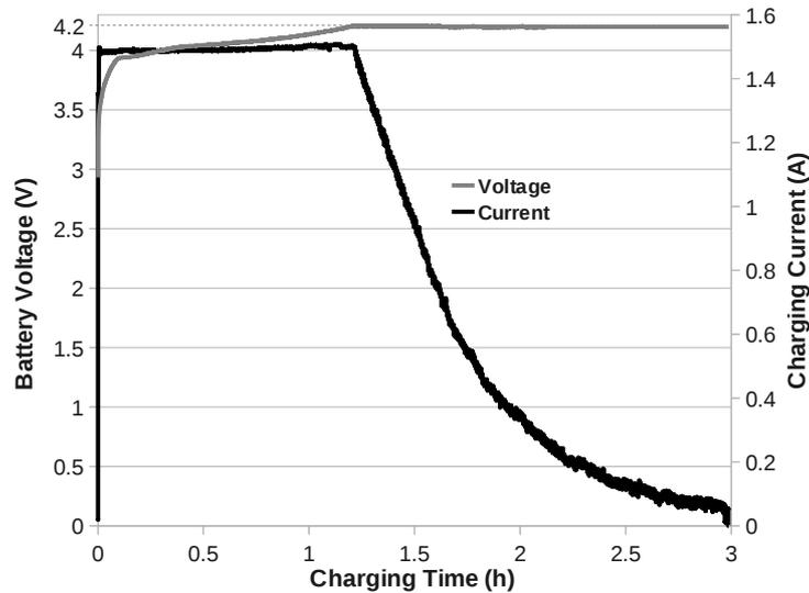
**Fig. 4.** CM1711ff current and voltage charge profile.
