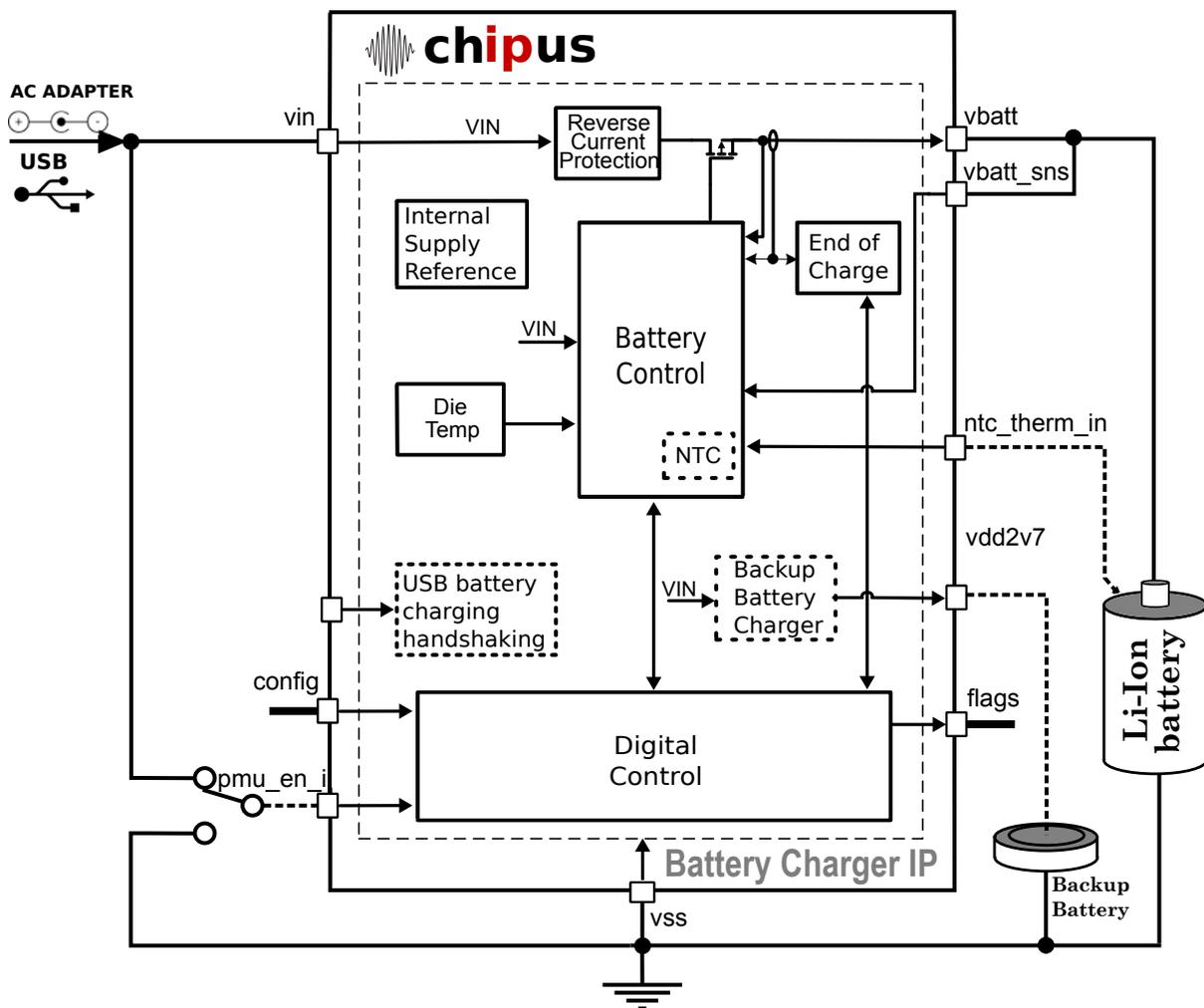
Fig. 1. Simplified block diagram for Chipus battery charger IPs.
