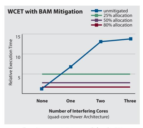
Figure 5: Worst-case execution timing stays steady after applying BAM
