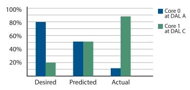
**Figure 2:** Example memory access bandwidth for DAL A and DAL C applications on different processors trying to access DRAM simultaneously.
