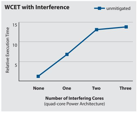
*Figure 4*: Worst-case execution timing varies with number of interfering cores
