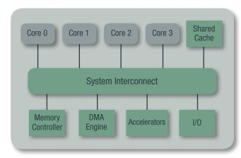
**Figure 1:** Separate processor cores (**gray**) share many resources (**green**) ranging from the interconnect to memory and I/O.
