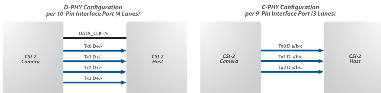
FIGURE 9 D-PHY and C-PHY lane configurations in the CSI-2 camera use case
