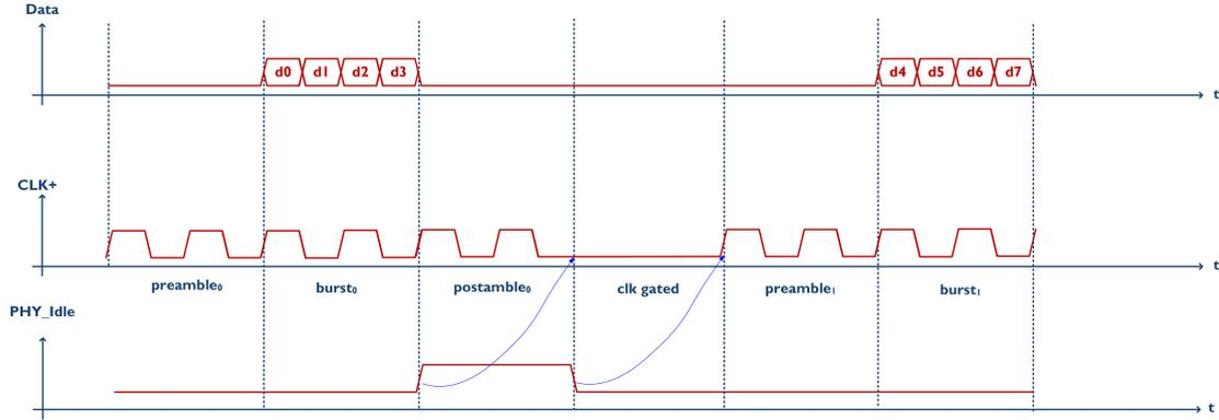
**Figure 17.** PHY\_Idle timing for entry/exit from clock gated state with  $M_{\text{ser}} = 4$  and  $N_{\text{par}}=1$
