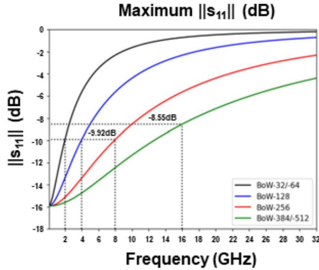
Figure 15. BoW RX Termination Maximum Return Loss
