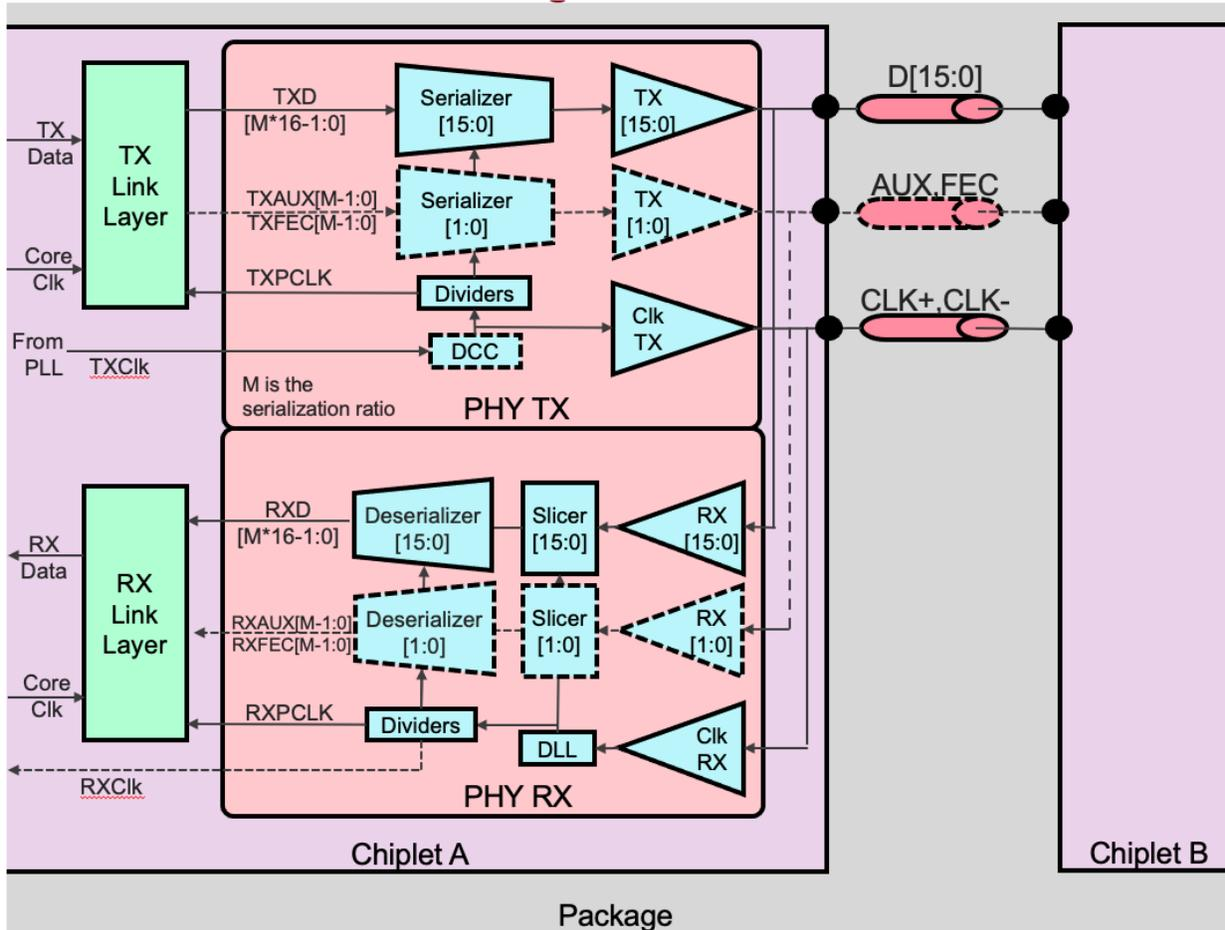
Figure 4. BoW Bidirectional slice block diagram
