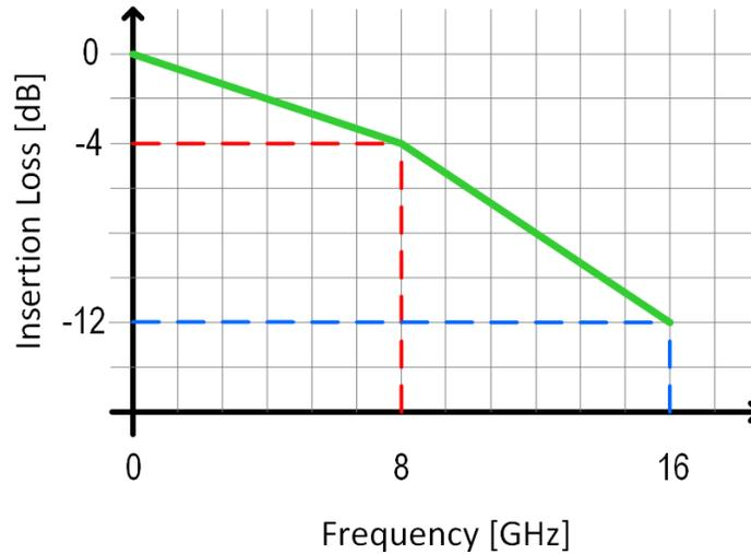
Figure 19. BoW Doubly-Terminated Wire Channel Loss Limit
