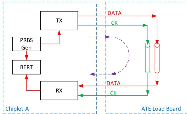
**Figure 25.** Long loopback testing
