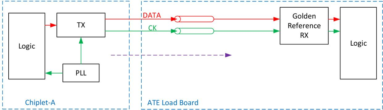
**Figure 22.** Open loop TX wafer test
