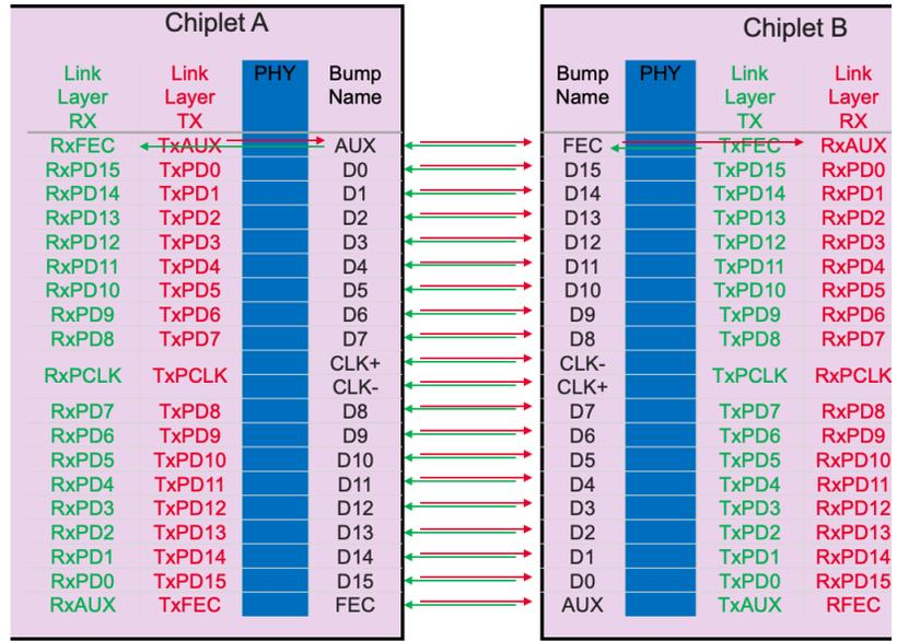
Figure 13. Alternating-Stacks Pattern of TX and RX Slices in a Link
