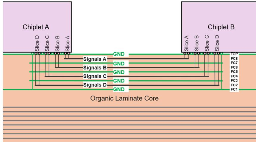
**Figure 10.** Cross section of a BoW Link in an Organic Laminate Package
