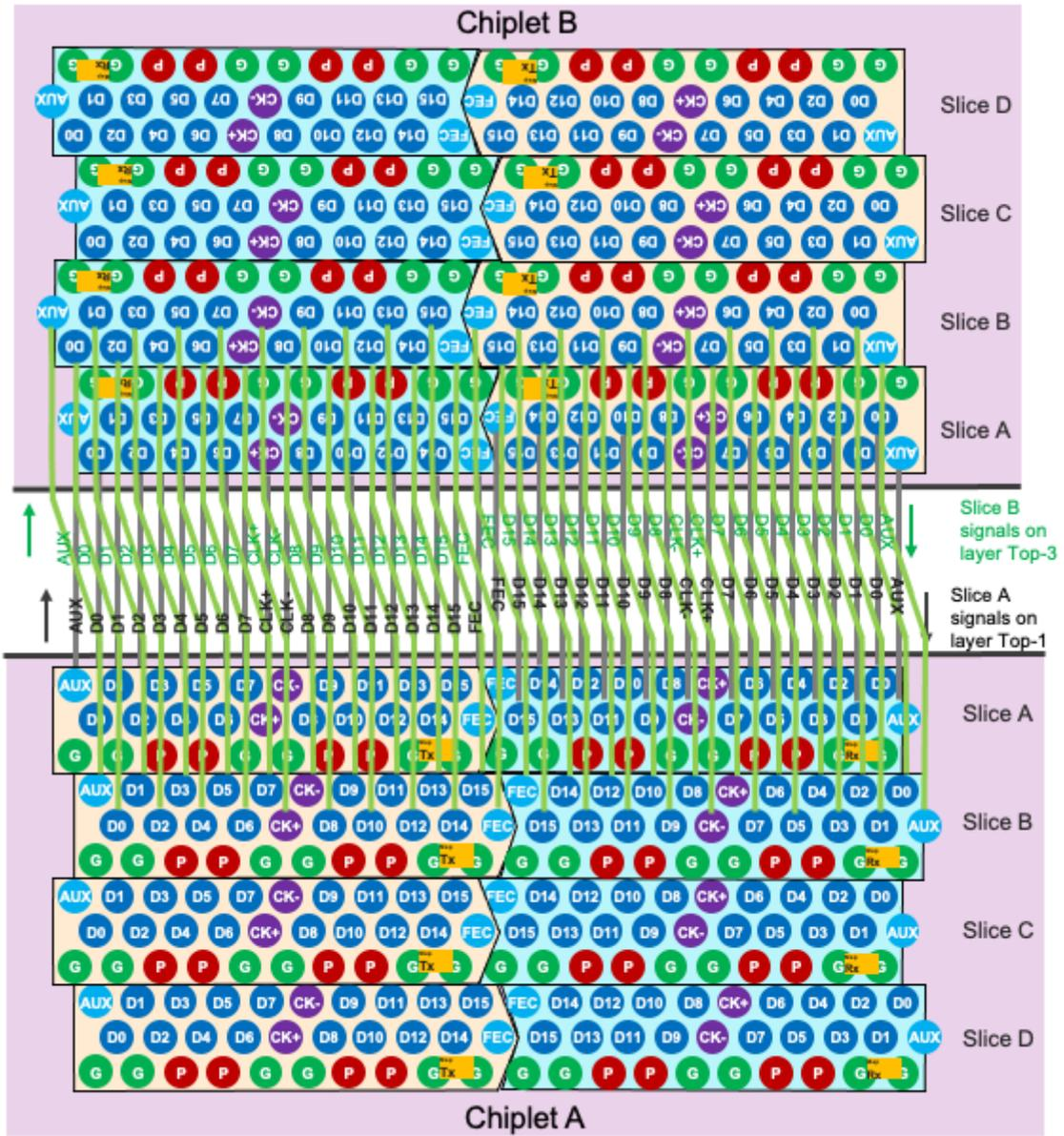
Figure 11. Staggered slices for the densest bump packing
