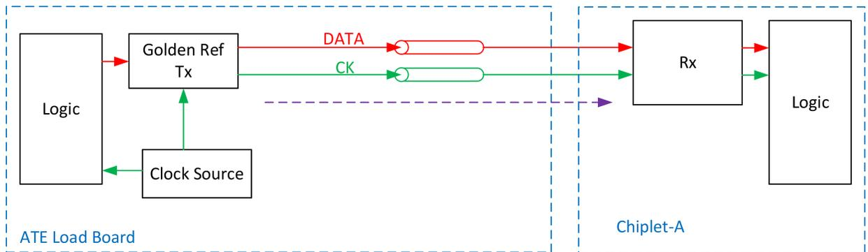
**Figure 23.** Open loop RX wafer test
