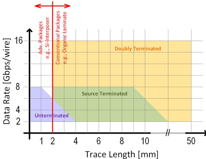
**Figure 2.** BoW Data Rate vs. Reach tradeoff
