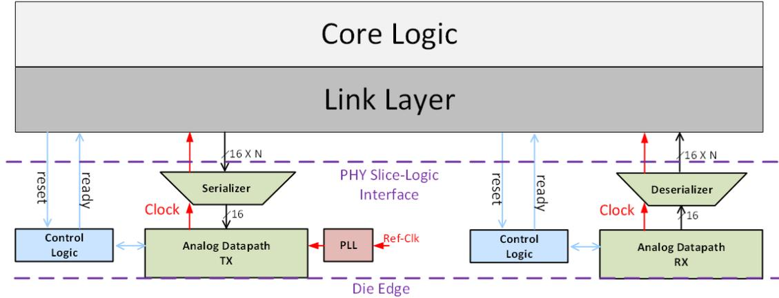
**Figure 3.** BoW slice logic interface
