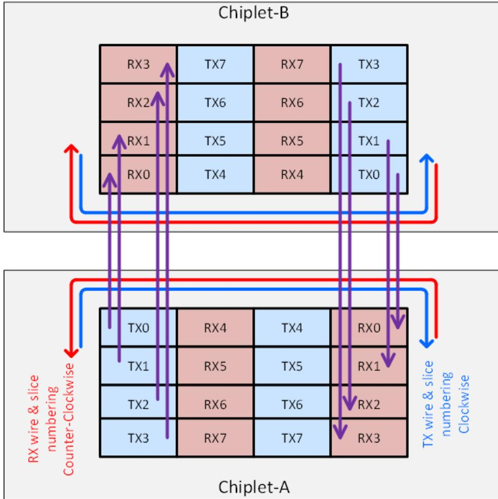
**Figure 12.** Alternating-Stacks Pattern of TX and RX Slices in a Link
