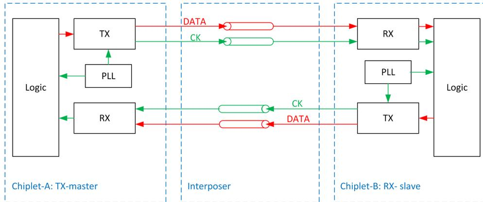
**Figure 26.** Chiplet-to-chiplet long loopback
