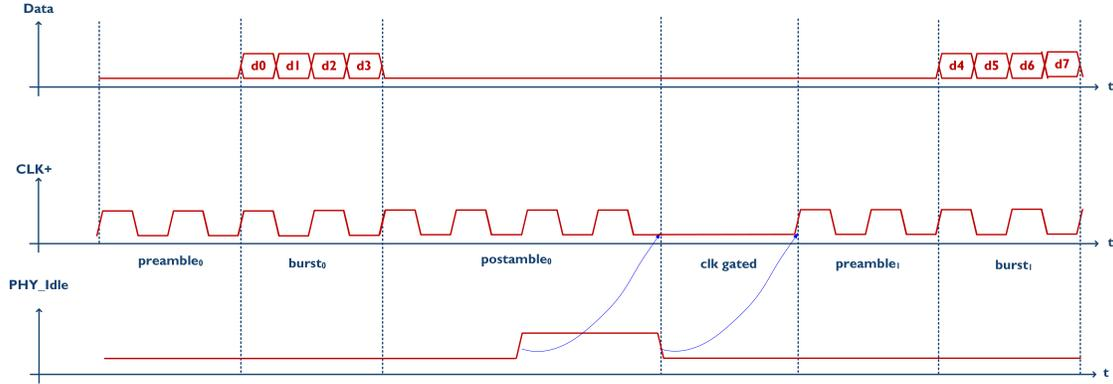
**Figure 18.** PHY\_Idle timing with  $M_{\text{ser,TX}} = 4$  and postamble  $N_{\text{par}}=2$
