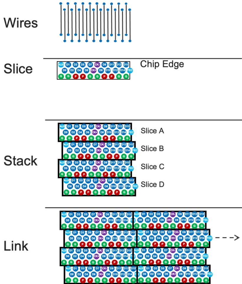
Figure 5. BoW Link Components
