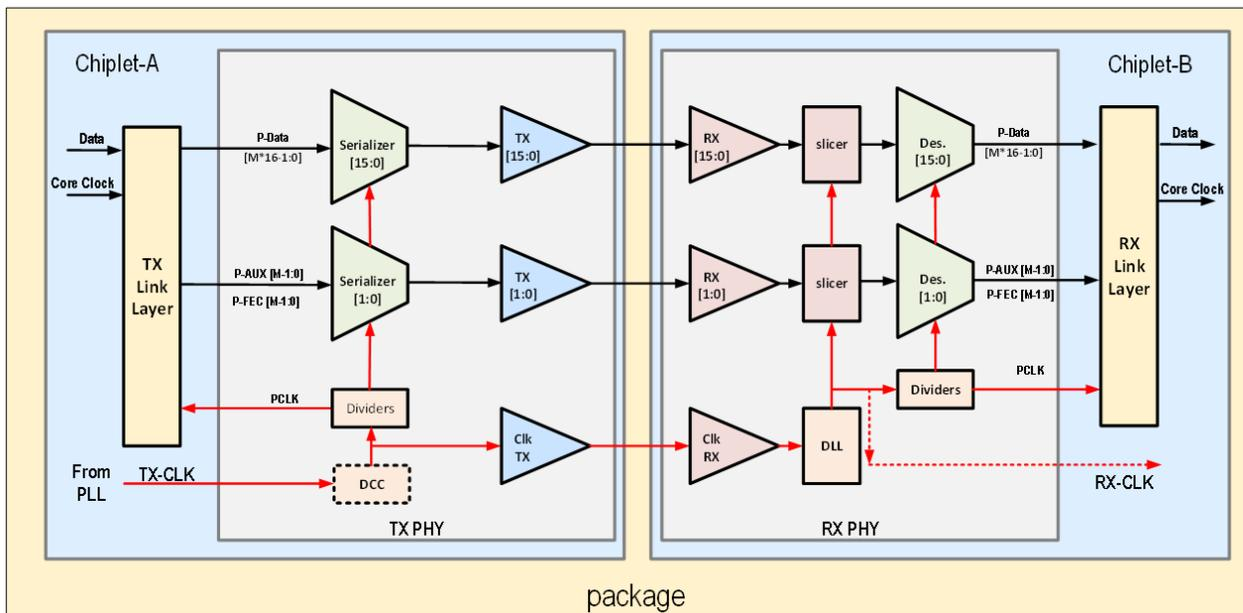
Figure 16. BoW Clock and Data Block Diagram - One TX Slice, One RX Slice
