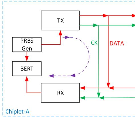
**Figure 24.** Short loopback testing
