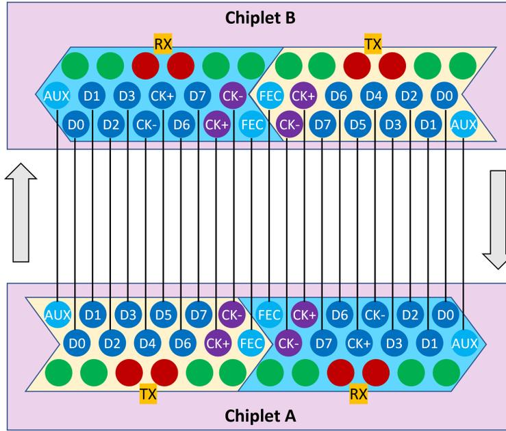
**Figure 8.** BoW Minimal Bidirectional Reference Half-Link
