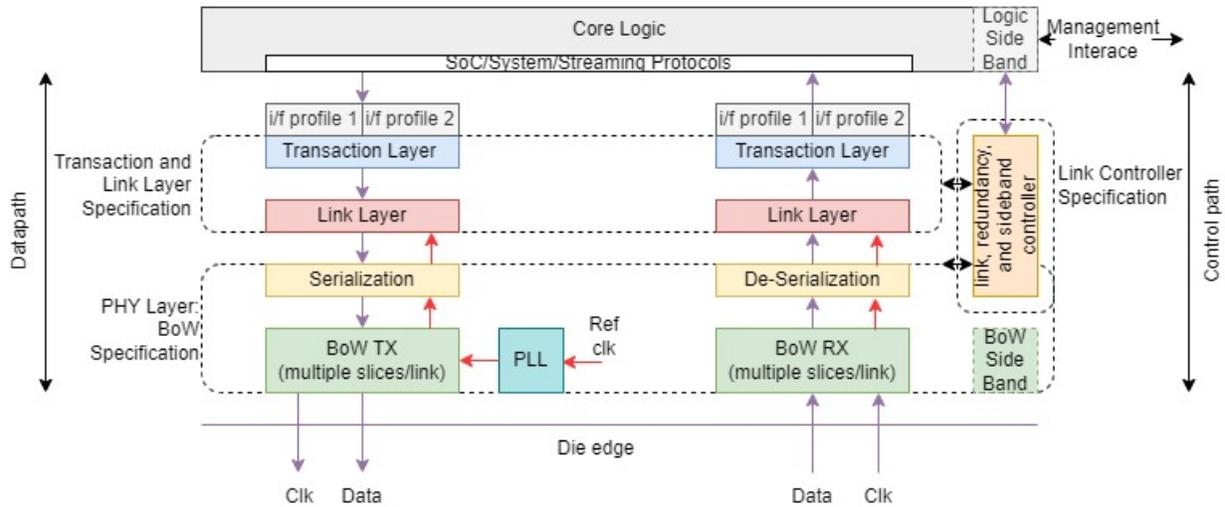
**Figure 27.** BoW link components: specifications and functionality
