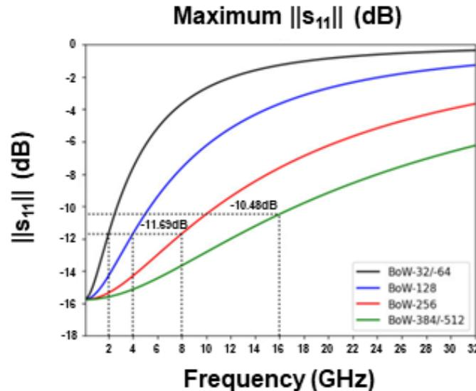
**Figure 14.** BoW TX Termination Maximum Return Loss
