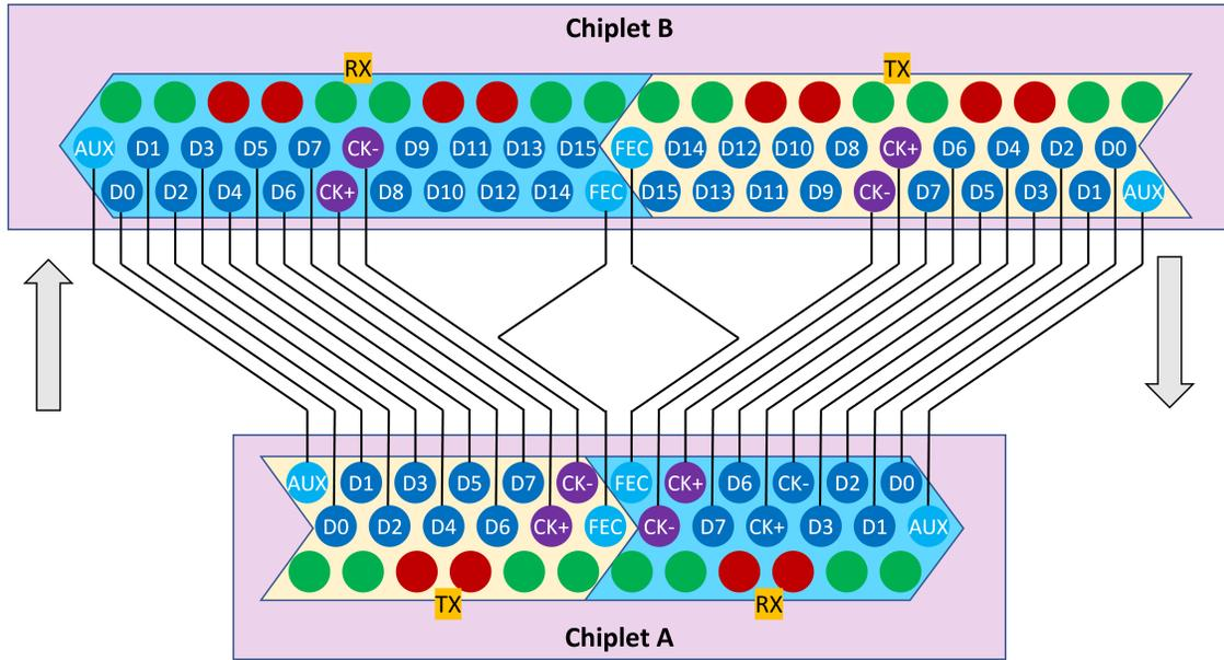
**Figure 9.** Reference Example of Half-Link to Regular Link Compatibility
